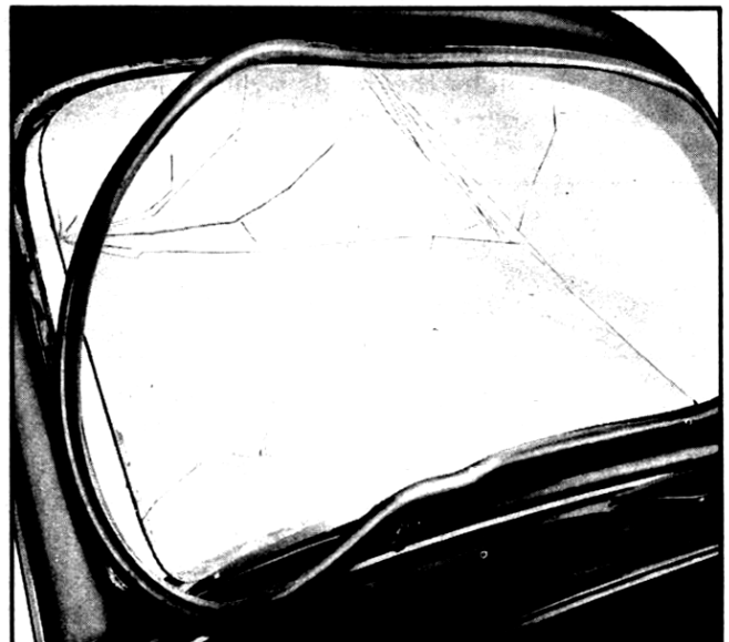
Fig. 3—Removing Glass from Weatherstrip
